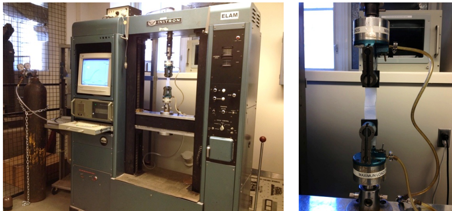
Figs. 7, left: Instron Universal Tensile Testing machine. Fig. 8, right: Detail of a silk specimen in the machine grips.
