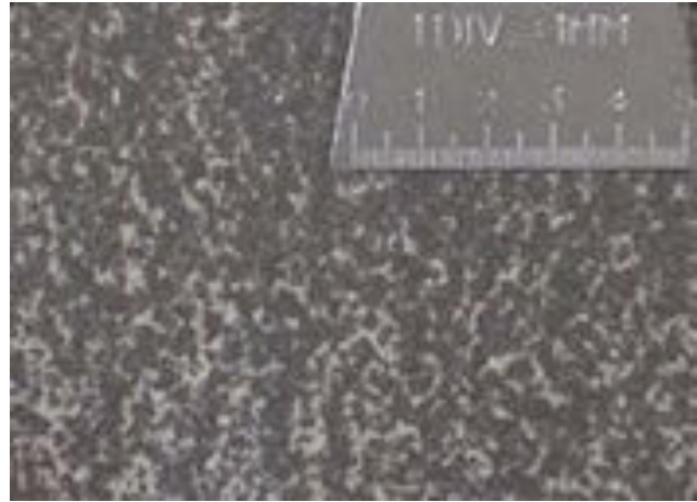
Figure 11. 40x Photomicrograph of characteristic ink reticulation pattern in a lithograph.
