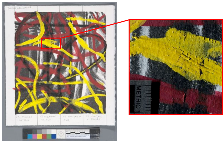
Figure 30. Mock-up for brush consolidation and detail of cleavage in the gouache paint film.
