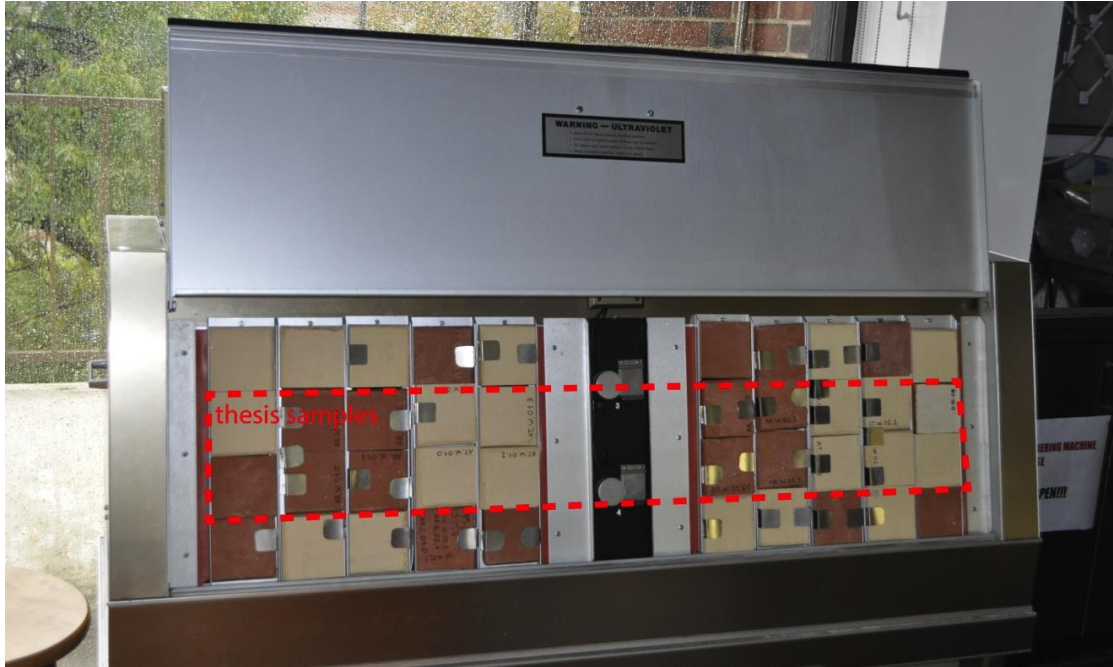
Figure 5: Pictures showing the samples in the weatherometer
