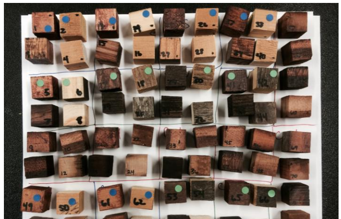
Figure 4. Treated 19mm cube samples arranged by jar number. Excluding the last row to the right, each set of four is (clockwise from upper left) kakishibu, raw juice, copper naphthenate, and untreated.
