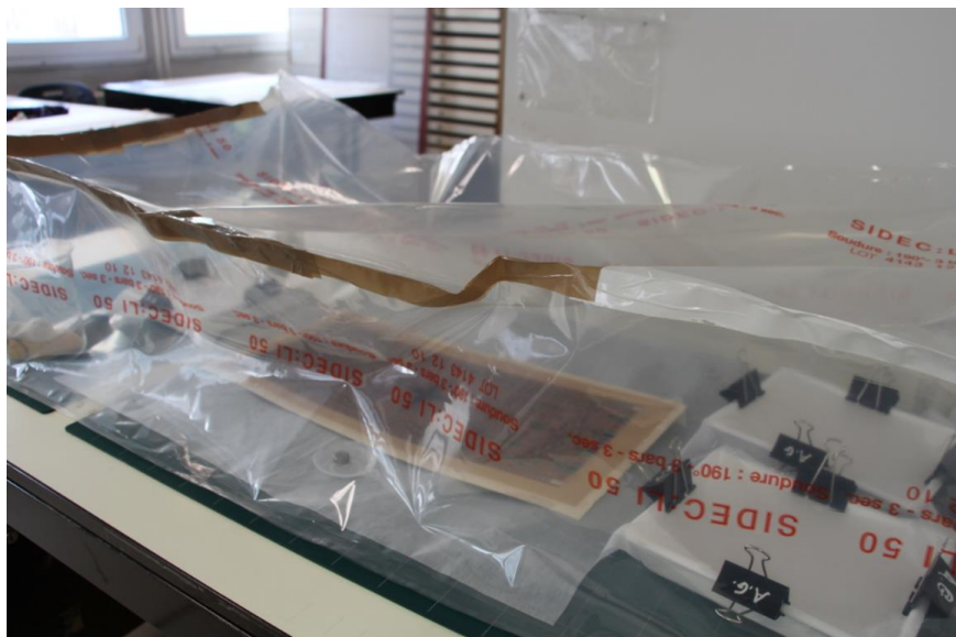
Figure 15: photography of the humidifying chamber in use
