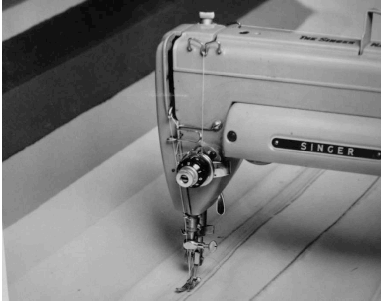
IMAGE A3.6 – The image at left is a detail of the sewing process. Though it is not visible in this image, Watherston recommended sewing straight stitch non-parallel, overlapping lines, for added strength.
