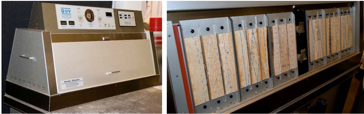
Figure 6. The QUV Weatherometer in the Architectural Conservation Laboratory both closed (left) and opened with specimen brackets inserted (right).
