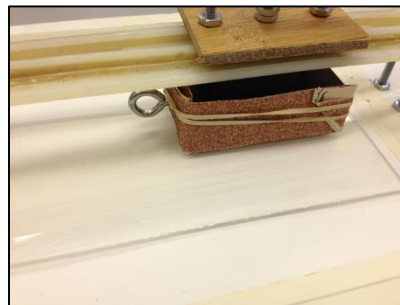
Fig. 9. Close up of scratching PMMA with rub-test machine
