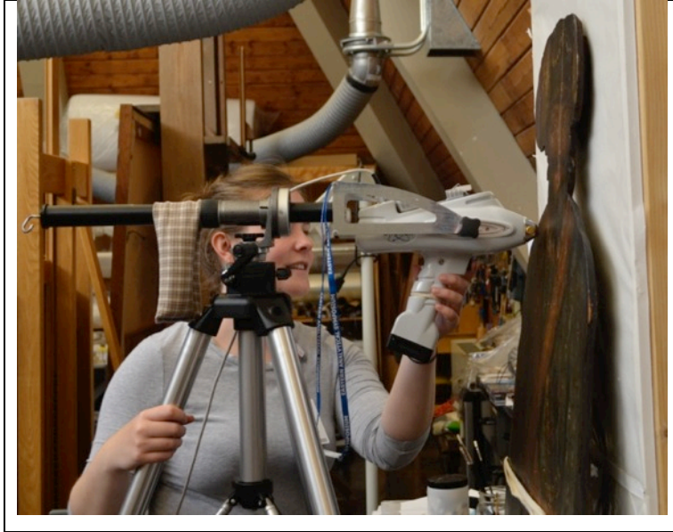
Figure 2. The author performing XRF analysis in the Winterthur Paintings Studio on the surface of the dummy board, ACP 1552, of a Turkish figure. Note the life-size scale of the object.
