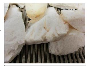
**Figure 11:** Delamination and active flaking of the cuttlebone.
