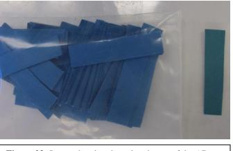
**Figure 23:** Image showing the color change of the AD strip after one week enclosure in the display case.
