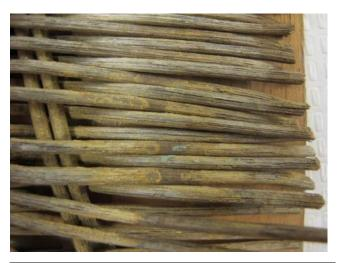
**Figure 7:** Showing the powdery yellow accretion, which may be remnants of paint from the former object.
