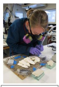
**Figure 12:** Applying .5% gelatin in deionized water to the surface of the bone with a nebulizer.
