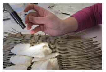
Figure 13: Detail showing micro-pipette consolidation of cuttlefish bone.
