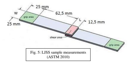
The ends of the samples were inserted into the grips of the tensile testing machine. The load was applied until the sample failed and the load and nature of the failure was recorded.
