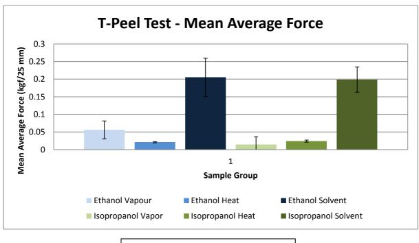
Fig. 9: T-Peel Test- Mean Average Force
