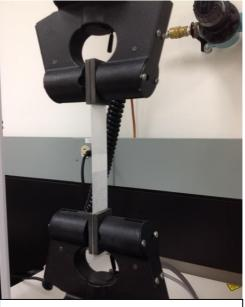
Fig. 4: LJSS sample in the tensile tester
