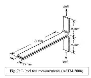
During testing, the unadhered ends of the samples were clamped in the grips of the tensile testing machine. The force was applied at a constant rate of 254 mm/minute (ASTM 2008). The peel resistance data was taken during the test as well as the nature of the sample failure.
