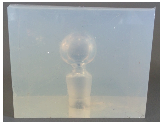
Fig 56. Clear silicone rubber mold made of the small glass decanter's stopper, ready to be poured with HXTAL epoxy.
