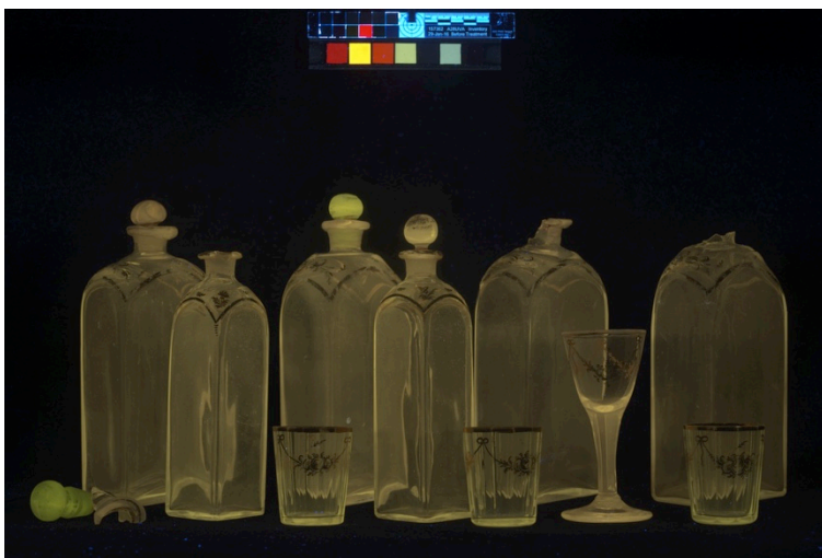
Fig 29. Glassware under UVA induced visible fluorescence. The yellowish-green hue is indicative of “potash” glass.
