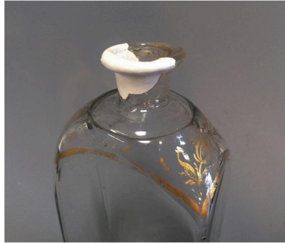
Fig 55. The plaster was shaped directly onto the glass over the wax and smoothed using various grit sandpaper.
