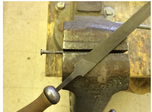
Fig 51. Filing rounded nails square to match the shape, length and width of the originals.
