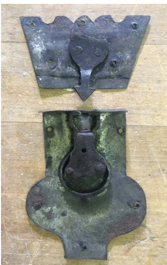
Fig 45 (left). The lock receiver stuck in its locked position, preventing the arrow from being inserted. Fig 46 (right). Two mild steel wedges are used to keep the lock in its unlocked position, allowing the lid to be closed.
