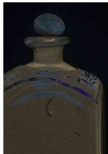
Fig 30. Decanter in UVC-irradiation. Note the blue fluorescence surrounding the gilding.
