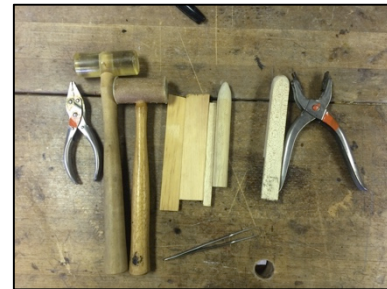
Fig 44. Distortions were corrected by hammering the metal between pieces of wood (on the left) and by using a number of other wooden tools with rounded tips (on the right)
