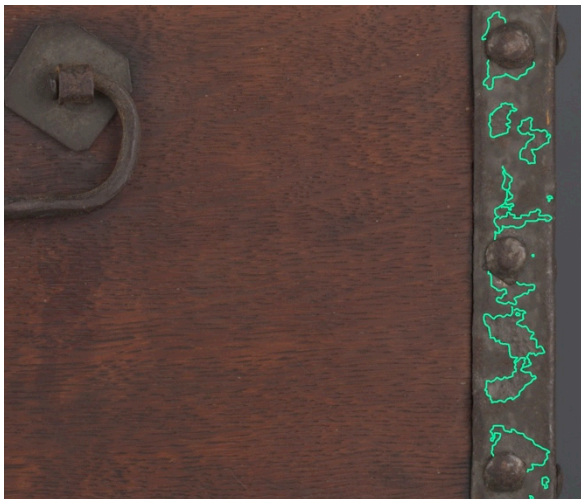
Fig. 21. The green outlines the scattered areas of a thin, degraded surface layer less than 1mm thick.
