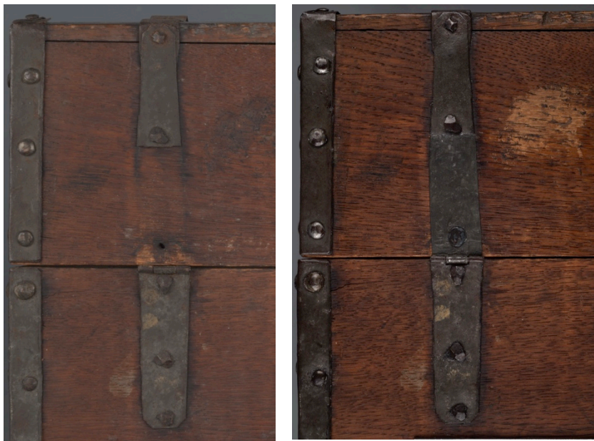
Fig 49 (left) and 50 (right). Back left hinge before and after treatment. The new, forged iron, replacement part (on the right) attaches the lid to the base and allows the case to be opened, closed.
