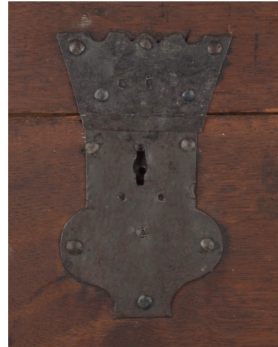
Fig 42. The lock mechanism darkened slightly after treatment with tannic acid.
