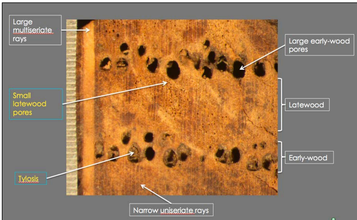
Fig. 26. End grain under magnification with different wood elements. Field size: 7.3 x 10.9mm
