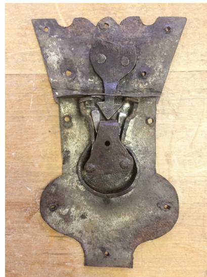
Fig 45 (left). The lock receiver stuck in its locked position, preventing the arrow from being inserted. Fig 46 (right). Two mild steel wedges are used to keep the lock in its unlocked position, allowing the lid to be closed.
