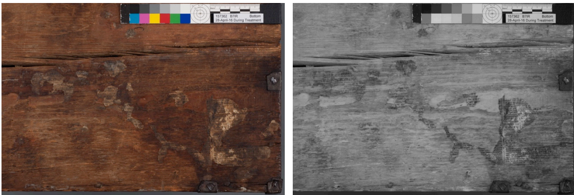
Fig 34-35. The newsprint on the base of the chest photographed in normal illumination (on the left) and in reflected near-infrared (IR) (on the right), in which the text is much more legible.
