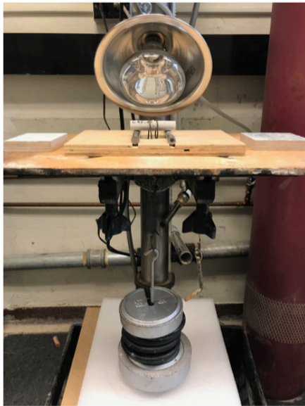
Stress - Creep Testing: Infrared lamp above the specimen and 20 lb. of weight suspended below.
