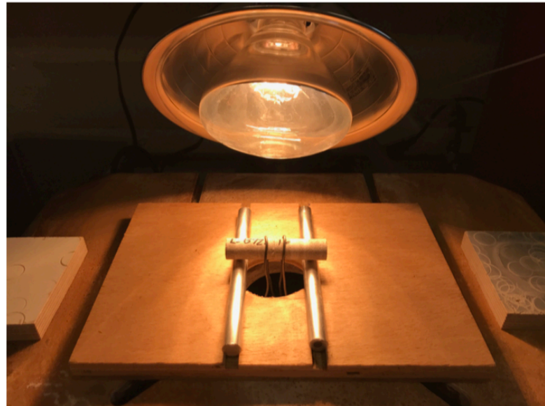
Stress - Creep Testing: Infrared lamp above the specimen and 20 lb. of weight suspended below.
