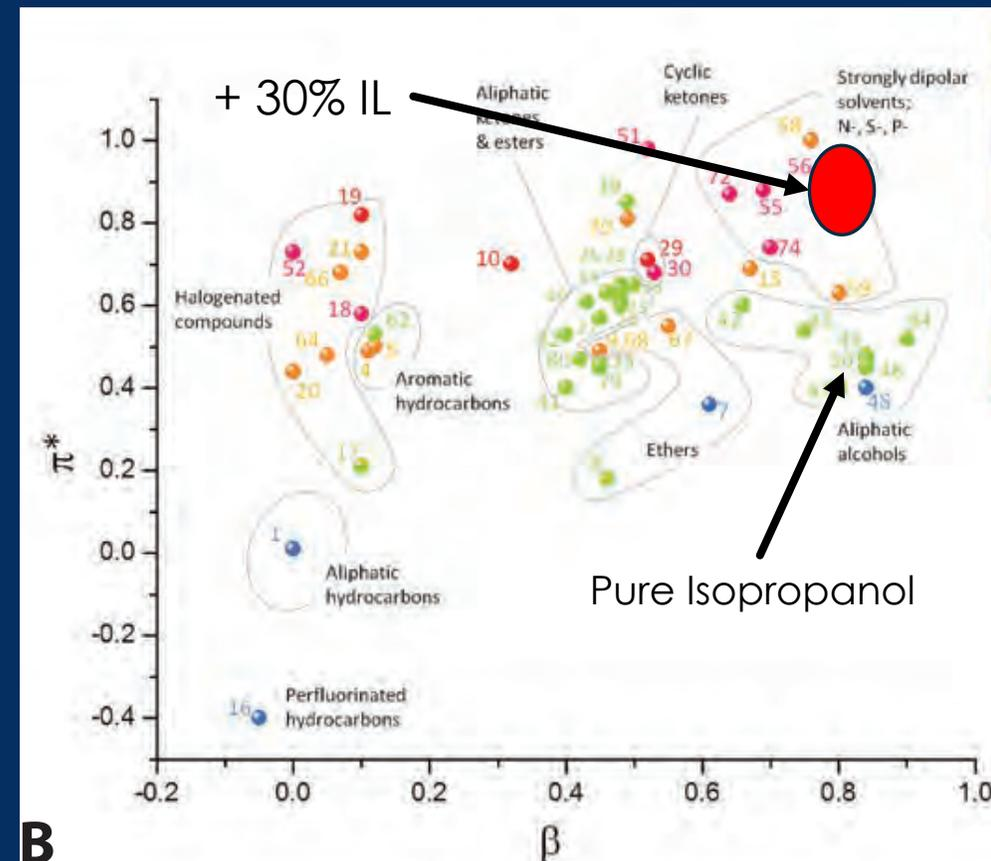
**Hypothesis: Binary mixtures of IL in isopropanol will solvate fresh and/or aged coatings of paint, varnish, and/or adhesives more effectively than isopropanol alone.**
