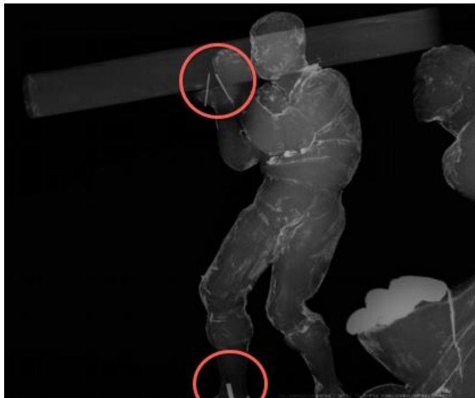
Fig. 20: X-ray of the figure holding the beam with pins in hands and feet circled. The join in the wheelbarrow is also visible.
