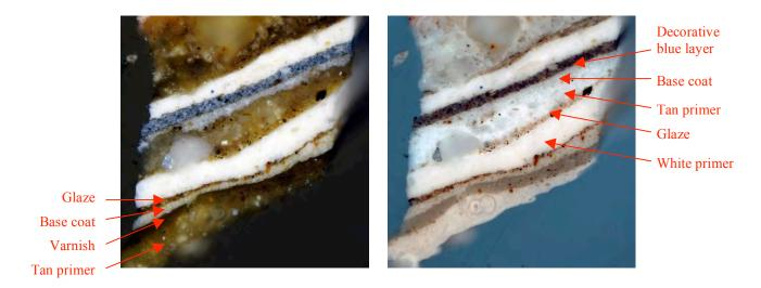
Figure 11: Sample from pilaster on corner cupboard, visible light and ultraviolet light, 400x magnification.
