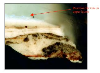
*Figure 7:* Sample from Stair banister Stained with TSQ, blue-violet filter cube 200x magnification
