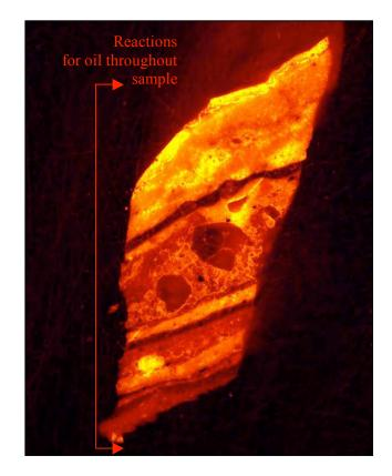
Figure 12: Sample from pilaster on corner cupboard, green filter cube, 200x magnification
