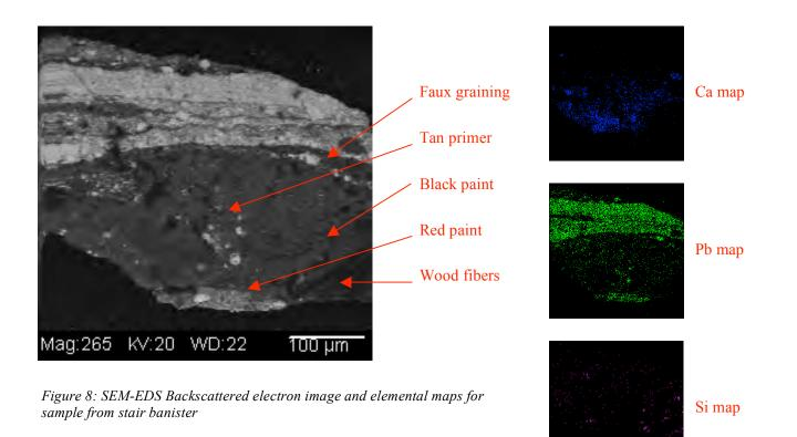
A spot analysis was done on the red paint layer with the SEM-EDS and this detected the presence of iron and lead. The lead may indicate the presence of red lead pigment, a lead dryer, or maybe a contaminant from the lead white paint layers above and below. The iron is likely to be red iron oxide pigments present in the layer. This was a cheap pigment that would have been in common use in the colonial period.
