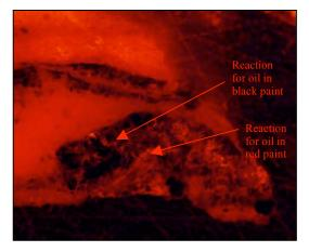
*Figure 6:* Sample from stair banister; Stained with Rhodamine B, green filter cube 400x magnification
