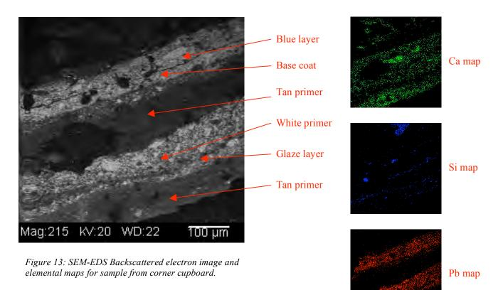
None of the blue paint layers tested with SEM-EDS detected any elements other than lead or paint fillers. Under magnification, the blue pigment particles are very fine and appear most similar to the iron containing pigment, Prussian blue, which was in common use at the time. Since Prussian blue has a high tinting strength, there may not have been sufficient concentrations of iron for it to be picked up by the SEM-EDS.
