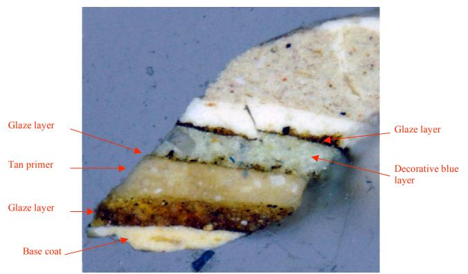
Figure 9: Sample from pilaster in Center Passage, visible light, 400x magnification.
