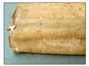
Broken sewing and torn vellum, typical of long stich sewing without backplates.
