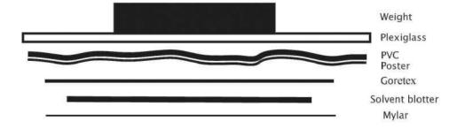
Fig. 10 Diagram of solvent vapour application
