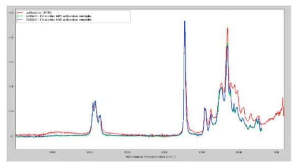
Fig 9. The adhesive being analysed (red trace) is compared to Filmolux 609 (green trace) and Filmolux 610 (blue trace), which have adhesives based on poly(2-ethylhexyl acrylate). Filmolux products are sold for use in document repair
