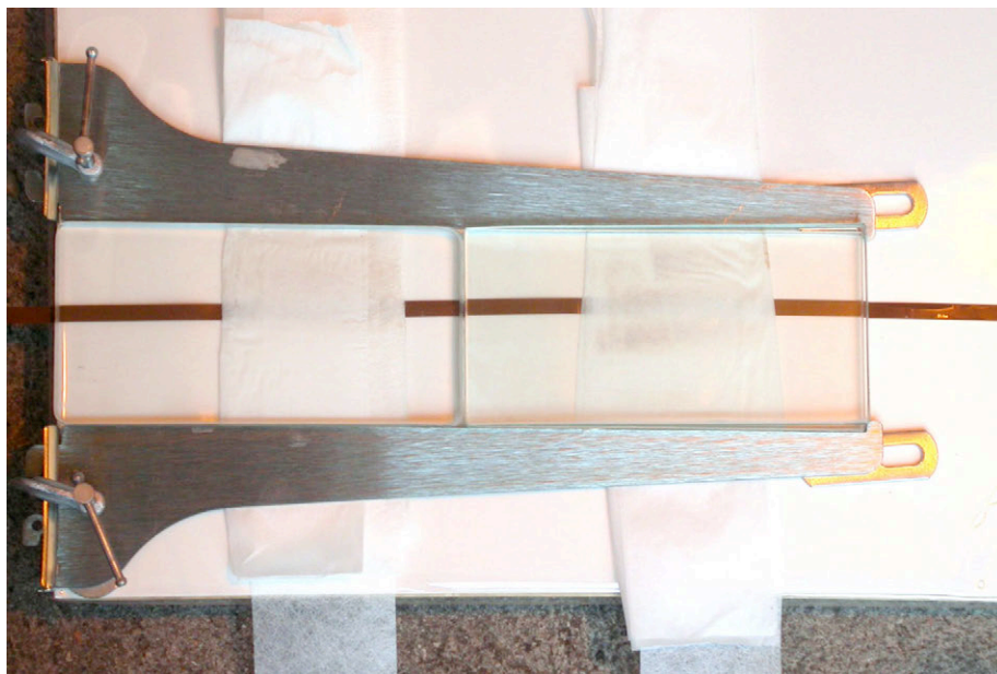
Figure 12. Top of cleaning platform showing solvent-saturated pads (left) and drying pads (right) beneath glass weights. The direction of audiotape travel is from left to right.
