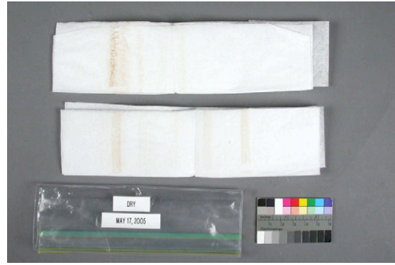
Figure 14. Drying pads following audiotape cleaning. Note heavier rust-colored offset on drying pads than on solvent-saturated pads.
