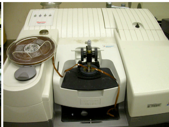
Figure 26. Close-up of the ATR attachment and pressure clamp holding the audiotape in place.
