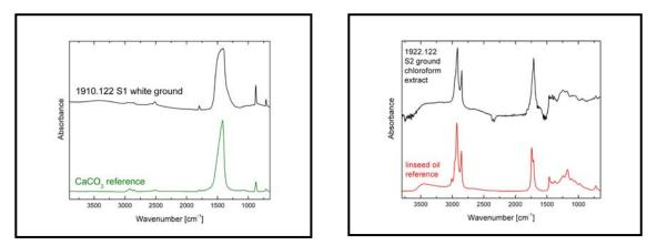
FTIR Spectra for ground samples 1 and 2
