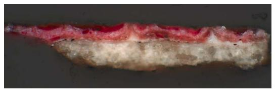
Cross section sample taken from the angel's robe Sample 20 x 2.5 magnification at capture
