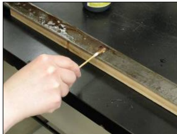
Fig.24 cleaning the surface of the blade
