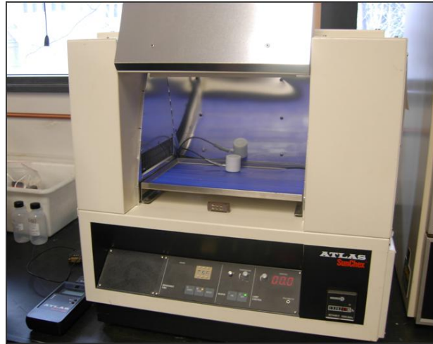
Fig. 11 - Atlas SunChex weathering oven with a xenon arc lamp.
