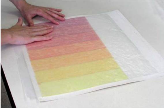
Pressing of Berg's drawing into contact with the adhesive sheet
