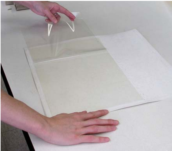
Removal of mylar from Lascaux 360 sheet
