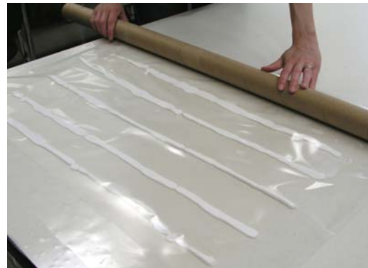
Lascaux 360 rolled between sheets of silicone mylar
