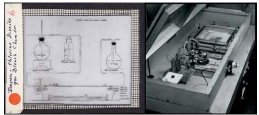
Fig. 4 Schematic drawing (left) and laboratory set up of chlorine dioxide gas bleaching chamber (right). ©Straus Center for Conservation, HUAM
