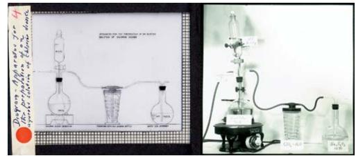
Fig. 3 Schematic drawing (left) and laboratory set up for infusing water with chlorine dioxide gas (right). ©Straus Center for Conservation, HUAM
