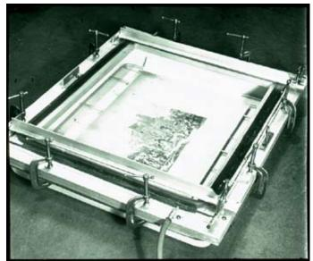
Fig. 5 Close-up view of the bleaching chamber with a print inside. ©Straus Center for Conservation, HUAM
