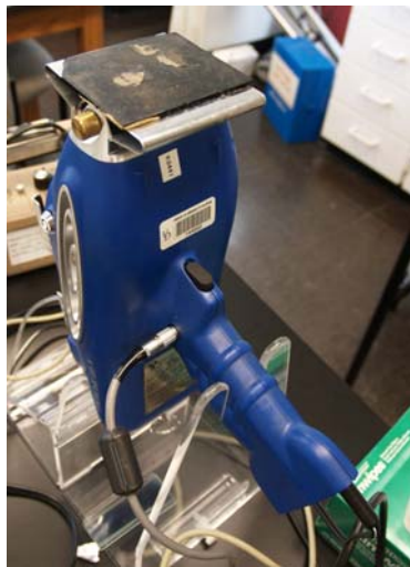
Figure 6: Each Ambrotype was Placed on the Stage and Analyzed with the Portable XRF
