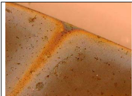
Figure 21: White Haze Due to the Scattering of Light by Silver Chloride Crystals; Reddish Orange Tarnish is Silver Sulfide Interference Colors
