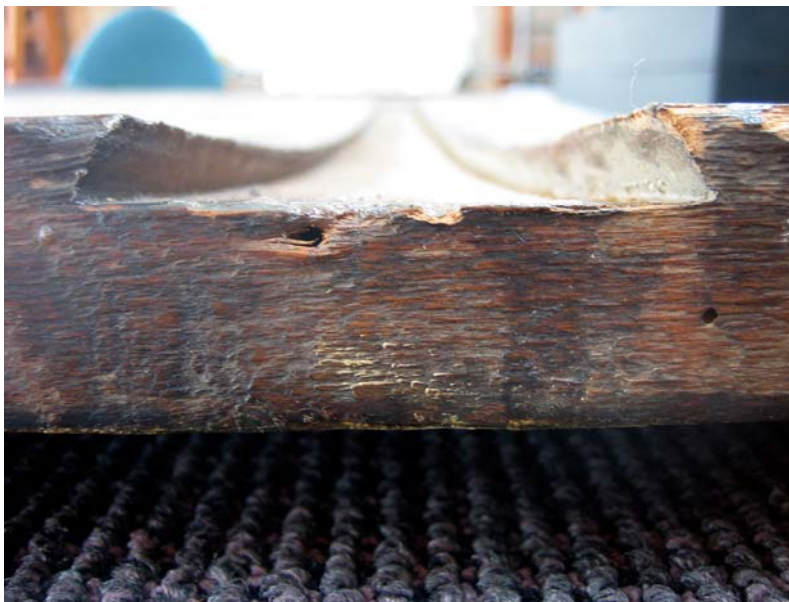
Figure 8: Trapezoidal cross-section (dovetail) of grooves in panel verso.
