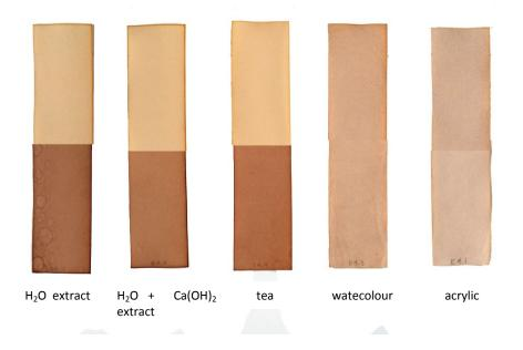
Figure 7 before aging images are above, after thermal aging images are below
