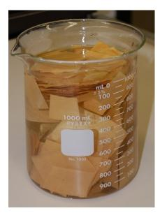
amount of discolouration removed. This step is illustrated in figure 1. After paper scraps were thoroughly saturated and wash water was discoloured the paper scraps were removed and the wash water was filtered and evaporated over heat. To prevent the material from scorching, once it had evaporated to a very dark concentrated liquid it was poured into a shallow tray and allowed to evaporate further until a solid material remained. This is shown in figures 2 and 3.
