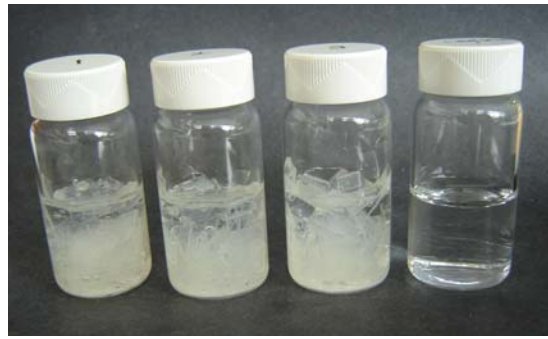
Figure 9: Control vial and test vials for pH testing with Butvar films
