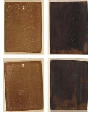
Figure 13: Before and after photos of coupon #25 not exposed to Butvar (top), and coupon #29 exposed to Butvar (bottom)
