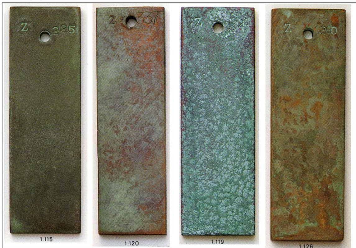
**Figure 12** Bronze coupons with applied nitrate patinas (Hughes *et al.* 1991).
