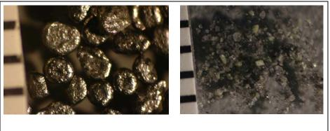
Figure 6:(Left) Photomicrograph of smokeless gunpowder. (Right) Photomicrograph of homemade black powder. Image: L.Horelick 2009.
