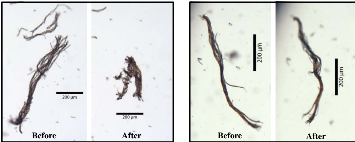
Figure 7: Corium fibers before and after shrinkage, unaltered (left) and altered (right).
