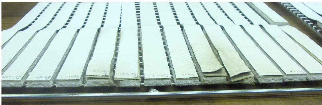
Figure 12. Moisture damage on bonded samples after ageing
