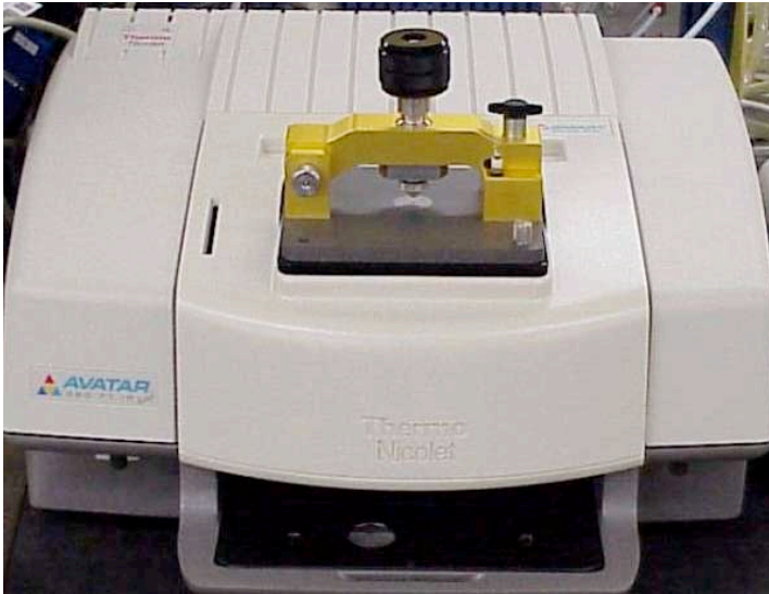
Figure iii. The Nicolet Avatar 320 FTIR Spectrometer with ATR Golden Gate attachment.
