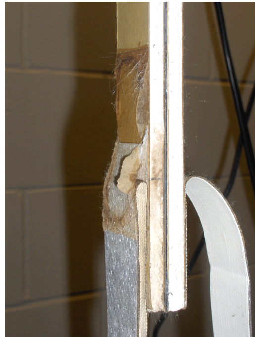
Figure 18. Example of separation issues observed during peel testing.
