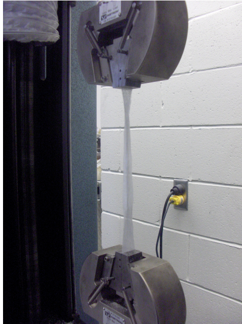
Figure 20. Necking and extended plasticity of the Reemay interleaf control samples during tensile testing.
