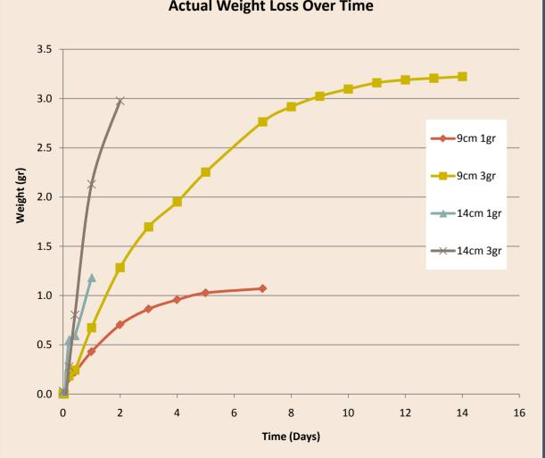
Fig. 3 Graph of sublimation rate of CDD aerosol spray. Actual weight loss over time
