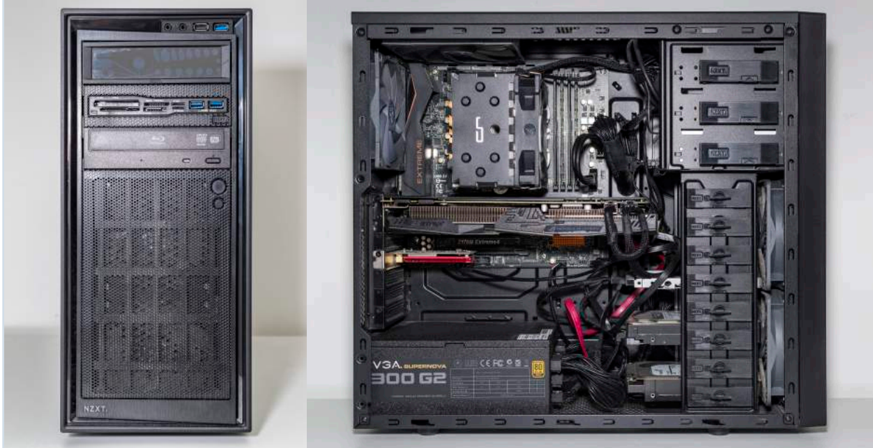
Figure 5-52. Workstation, front view. Figure 5-53. Workstation, internal view.
