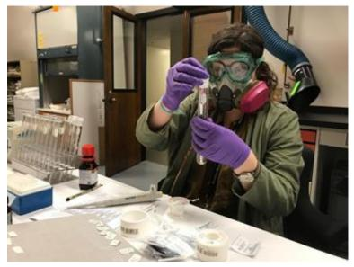
Fig. 2. Preparing textile samples to be exposed to linalool prior to artificial aging
