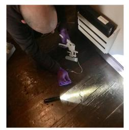
**Fig. 5.** The raking light makes the mercury drips more visible to cleanup with a specialized mercury spill kit
