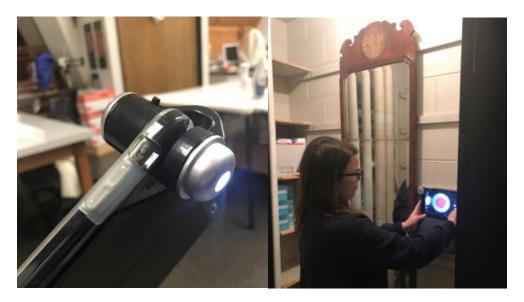
**Figs. 8,9.** The microscope attaches to the iPad and provided consistent lighting and a fixed focal point for the photographs of the sensors
