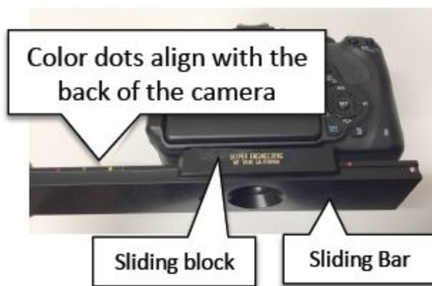
Fig. 13: Sliding bar with alignment dots and camera sliding block labeled. Image: JJ Chen, Creating Stereo Pairs with Stereo Slider Bar handout, 2018.
