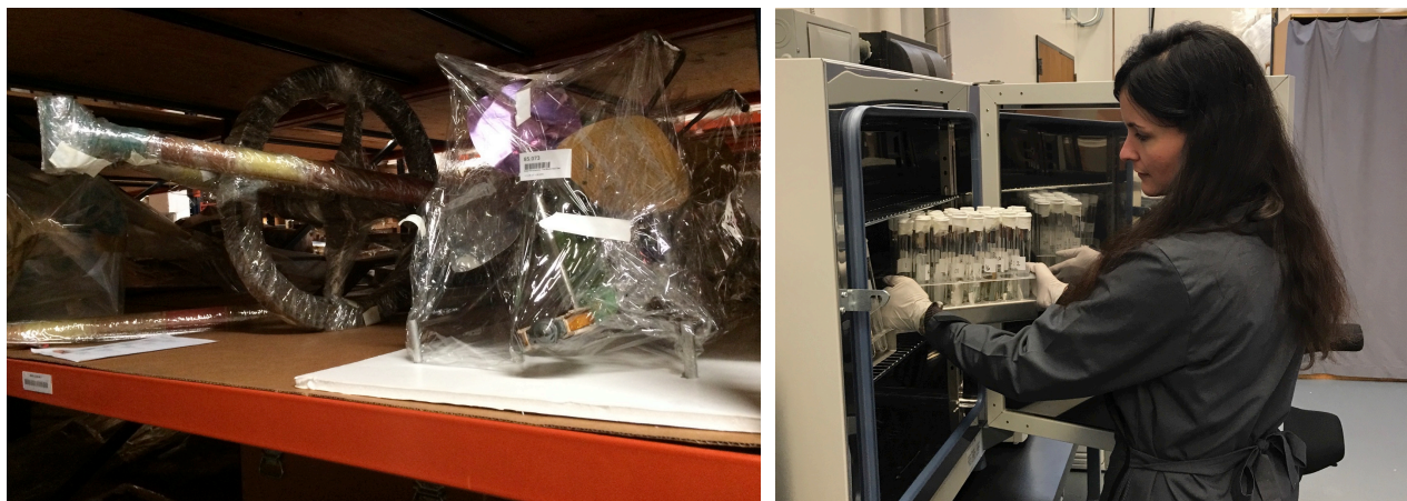
Figures 6, 7 – (left) Dartek-wrapped objects in storage at the RRF. Image courtesy Jennifer Myers; (right) Jennifer performing one step in the Oddy Test protocol. Image courtesy Melissa King.
