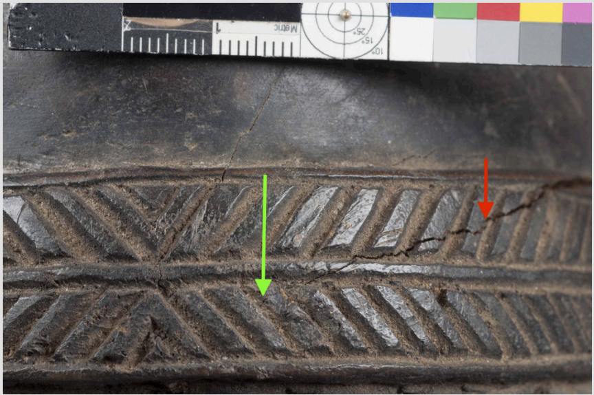
Propagation of a crack at the top of the head, near the center of the growth rings
