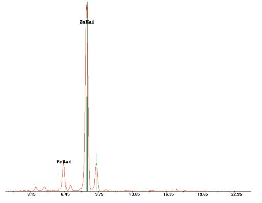
Figure 3. XRF spectrum, in keV, of join, diagonal off-white metal on base, Side C. Lead-tin solder, zinc chloride flux and putty with titanium white and calcium-based filler.
