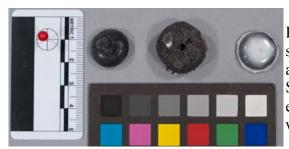
Elite Double 8 silicone rubber mixed with strontium ferrite powder (left) and iron filings (middle). Silicones Inc. P-4 silicone rubber mixed with equal parts strontium ferrite powder and chalk white (right).
