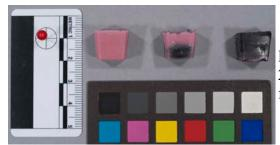
Elite Double 8 silicone rubber (left) mixed 2:1 (middle) and 1:1 (right) with strontium ferrite powder
