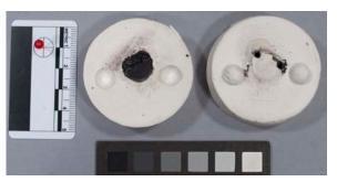
Plaster mold with bonded magnetic coating
