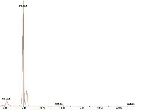
Figure 2. XRF spectrum, in keV, of the light green coated metal, Side A. Photo
