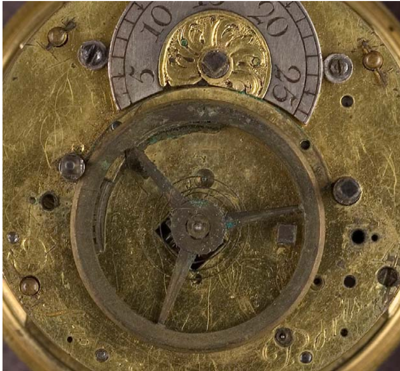
Figure 26, DuFresne, Paris, 1698. Original late-seventeenth-century spring balance
