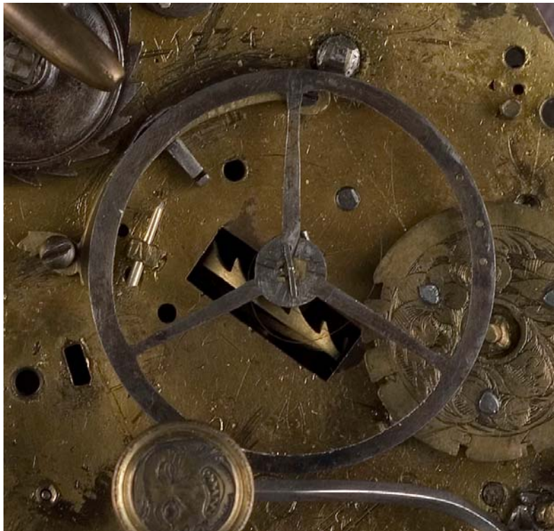
Figure 27, Buffalo Scheirer clock. Spring balance adapted from foliot during the late seventeenth or early eighteenth century
