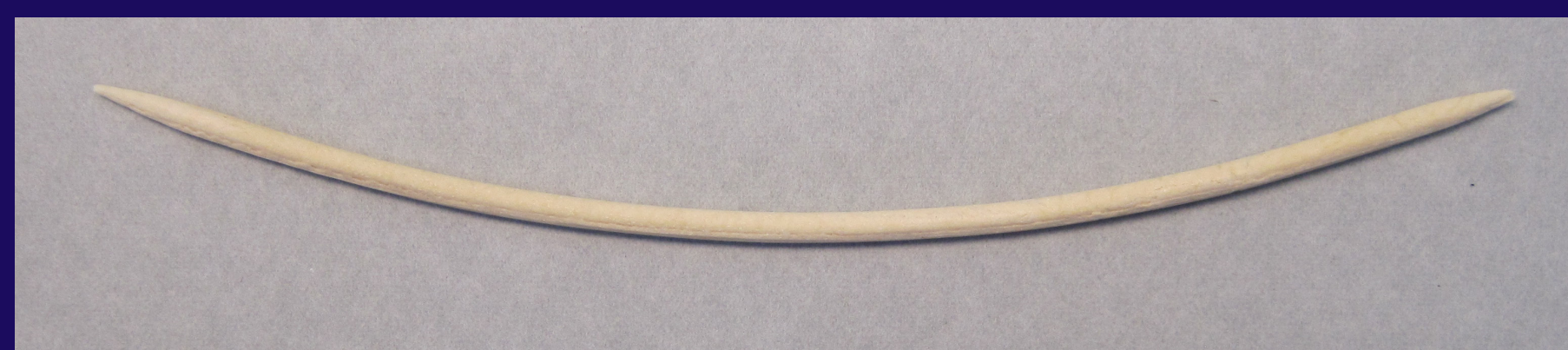
Molded Lascaux rods are flexible and will hold their shape.
