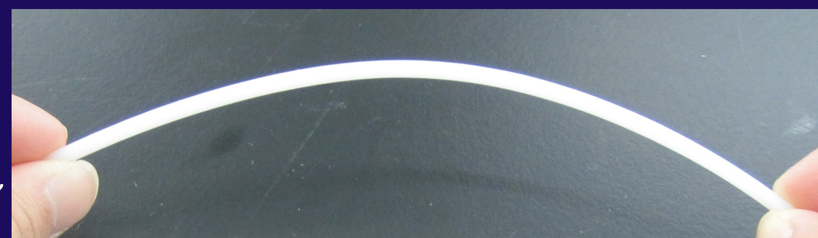
Above: Friendly Plastic and InstaMorph are two inexpensive brands of PCL pellets. Right: Molded PCL rod, showing flexibility.
