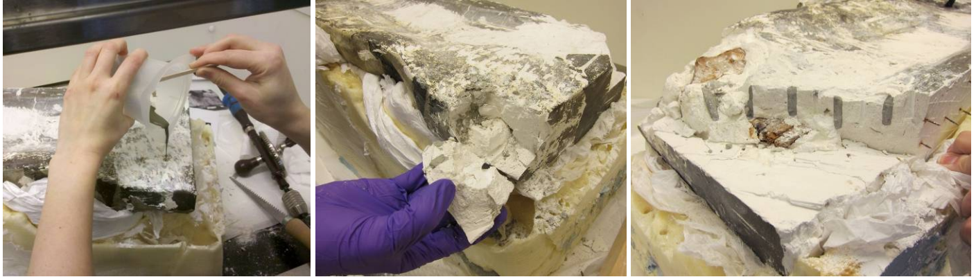
From left to right, Figure 20: filling expanding hole with Dexpan water slurry, Figure 21: first chunk of plaster removed; Figure 22: plaster removal in progress
