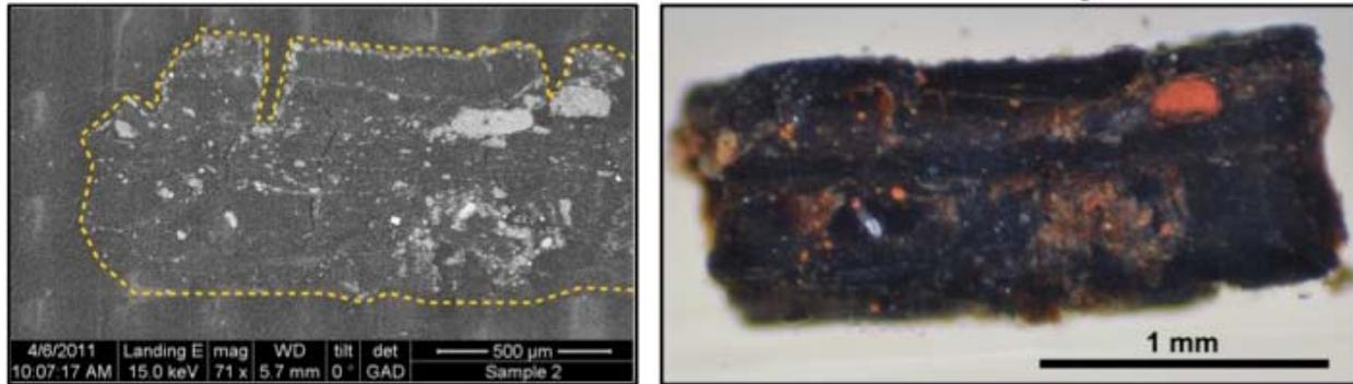
**Figure 14:** Left image is was taken with variable pressure scanning electron microscopy both with a back-scattered detector. The right image is a visible light photograph of the same sample.
