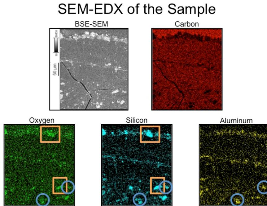
**Figure 16: SEM-EDX maps for a detail of the sample from X86.385. The orange rectangles identify Silicate particles and the blue circles mark alumino-silicate particles.**
