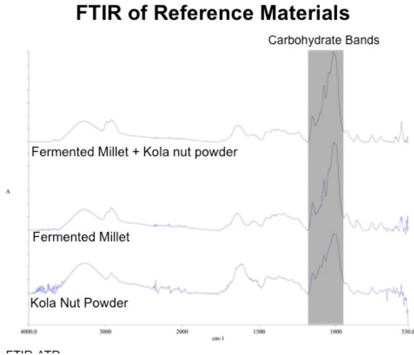
**Figure 10: Graph of the FTIR data for the Millet and Kola Nut reference material. There is no way to consistently differentiate between the two materials using this technique. The analysis was done with a Perkin-Elmer Spectrum One infrared spectrometer in Attenuated Total Reflectance mode with a Zn-Se crystal.**
