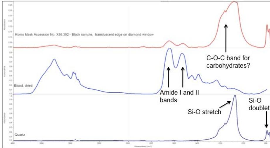
**Figure 11: Graphs of the FTIR data for a surface sample (red) as well as a blood (light blue) and quartz (dark blue) standard. Analysis completed with a Hyperion 3000, ATR Diamond 80 micrometer facet.**
