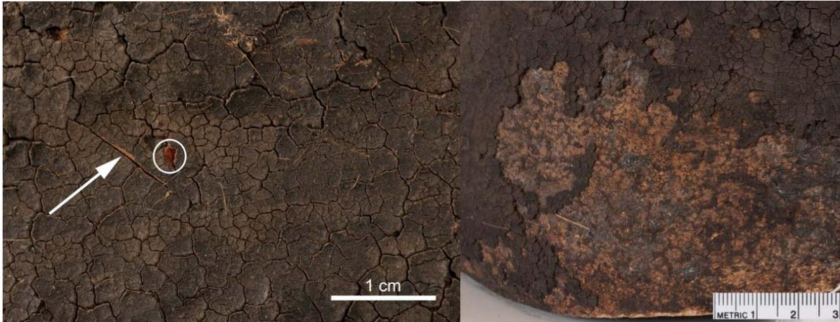
**Figure 2: Details of the surface from X86.385. Left image shows a red particle (circled) and a plant fiber (arrow) embedded in the surface. Right image shows an area of loss that reveals the wood beneath.**
