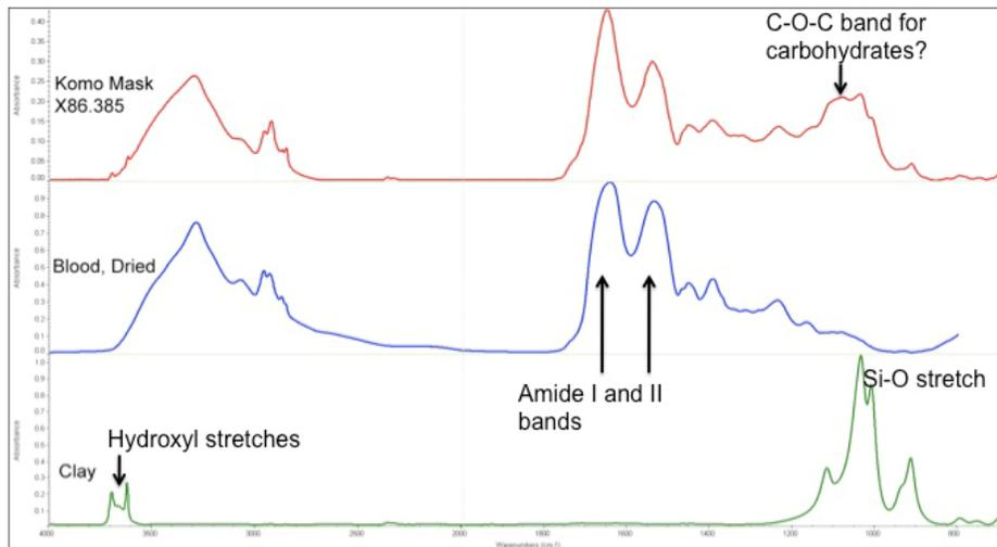
**Figure 12: Graphs of the FTIR data for a different area of the same surface sample (red) as well as a blood (light blue) and a clay (green) standard. Analysis completed with a Hyperion 3000, ATR Diamond 80 micrometer facet.**
