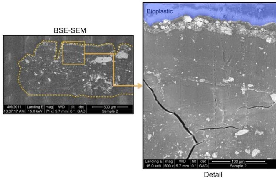
**Figure 15:** The left image shows the overall view of the sample, with the location of the detail marked with an orange rectangle. The right image is the detail with the mounting resin (Bioplastic) shown in blue.
