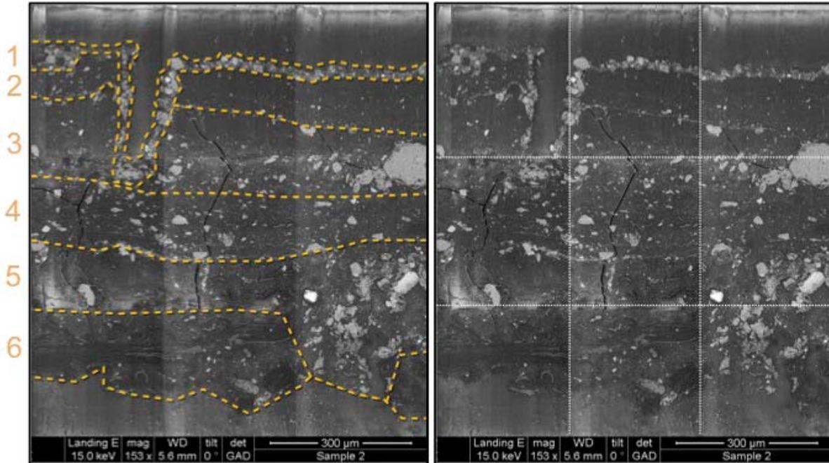
**Figure 17:** Image of a larger detail from the sample from X86.385. The orange dotted lines in the left image show the possible layers and the white dotted grid lines in the right image show the borders between the smaller images that were stitched together to form this larger image.
