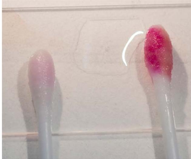
**Figure 9: Positive results for Kastle-Meyer blood test. The positive control is animal blood. Color developed within 30 seconds.**
