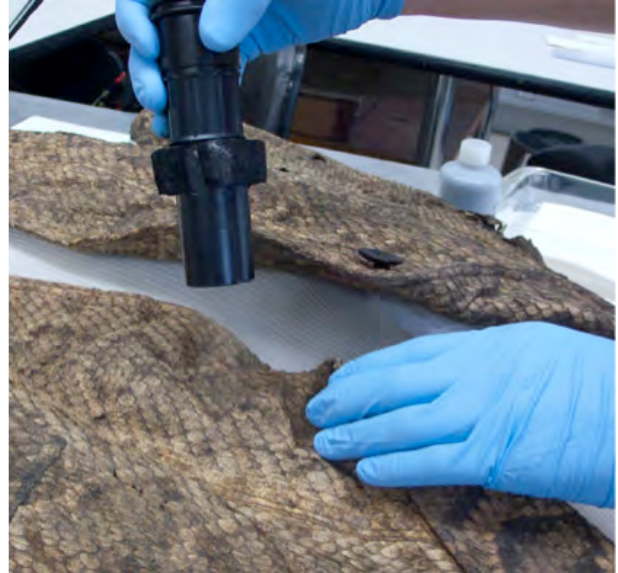
Figure 35: Application of local humidification using the ultrasonic nebulizer wand. Although not pictured, a blotter paper was wrapped around the tip of the wand to prevent dripping.
