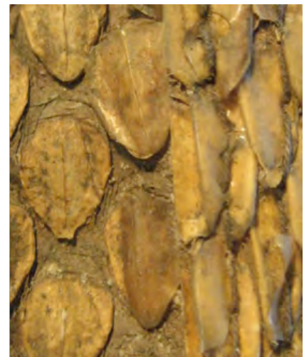
Figure 36: A scale before (left) and after (right) reattachment of the keratinous scale with BEVA film. The color of the area with the missing scale on the left is lighter.
