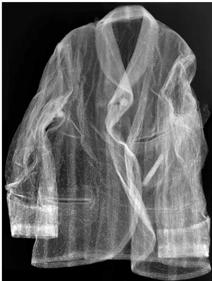
Figure 19: X-radiograph (25 kV, 25 mAS (50 seconds, 10mA), 55"FFD, with an 8-ply mat board for filtration)
