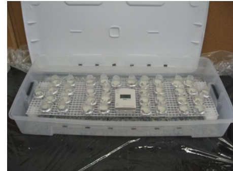
Fig. 7. Chamber set up with sample assemblies on the grate and data logger in the center of the chamber.
