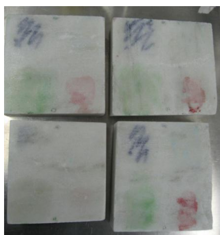
Fig. 31. Samples after graffiti removal Top left: CeNano Top Right: Nanopool Finish Bottom Left: Nanopool AntiGraffiti Bottom Right: Control
