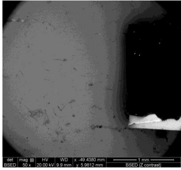
Fig. 19. CeNano Portol Pro: tape lines were not as easily distinguishable in comparison to the other products. Potentially not enough product applied.
