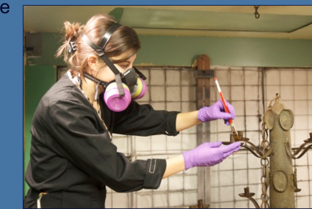
Courtney applying the inhibitor in the spray booth for adequate solvent extraction.
