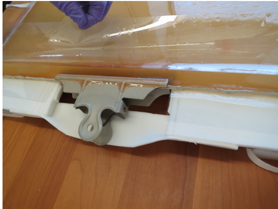
Fig. 16: Images of discolored (reddish) pooled plasticizer on back clip
