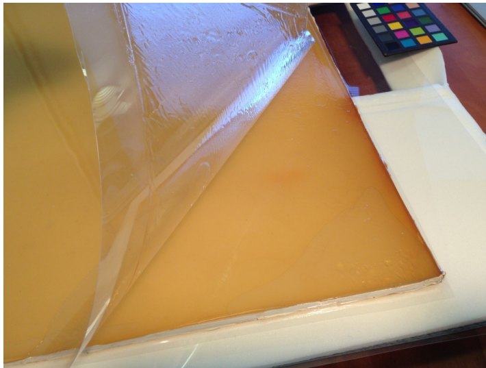
Fig. 5: Images showing pooled plasticizer below Mylar on front surface of 1995.265
