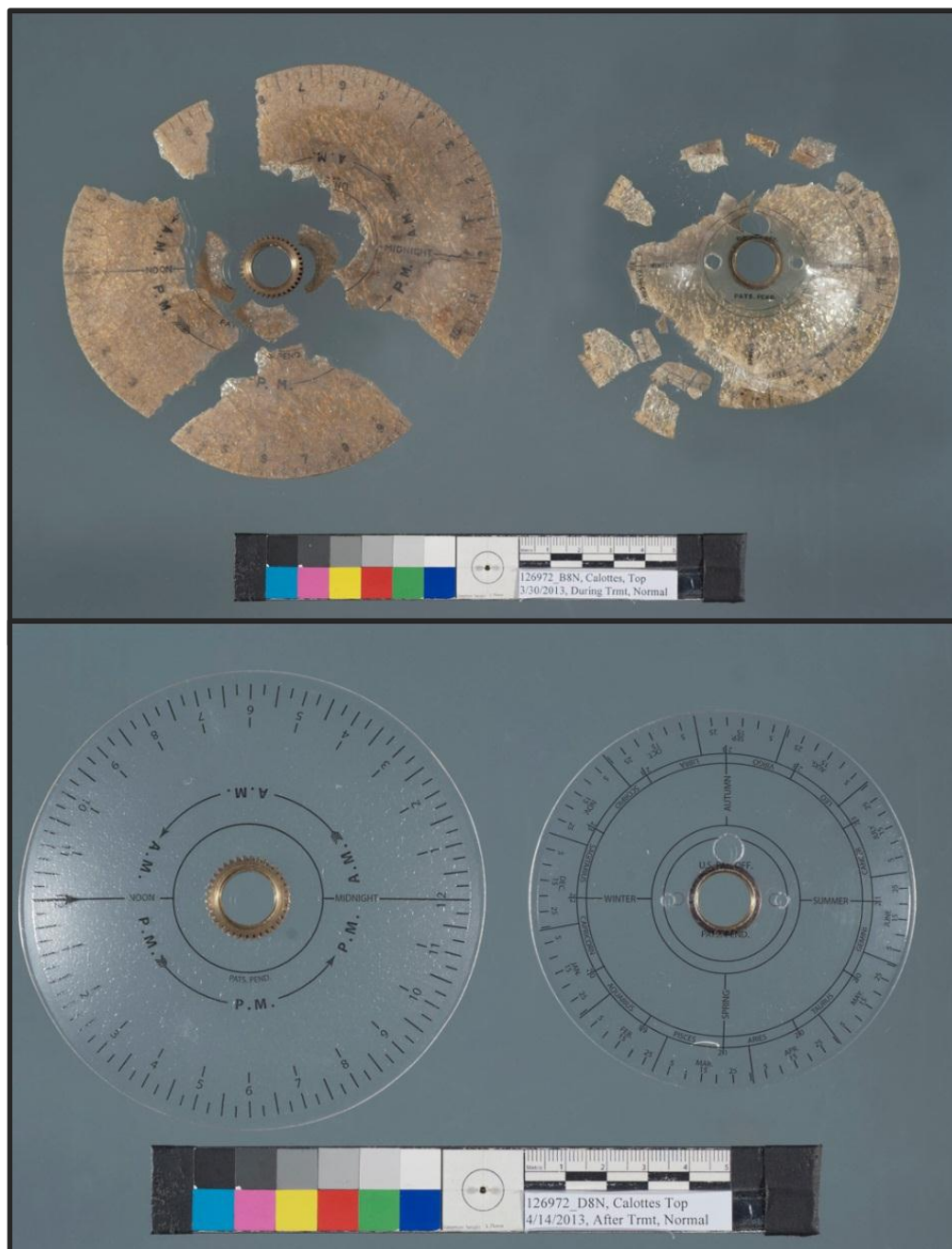
Figure 44: The original, degraded cellulose acetate calotte discs (upper image) compared to their PMMA replacements.
