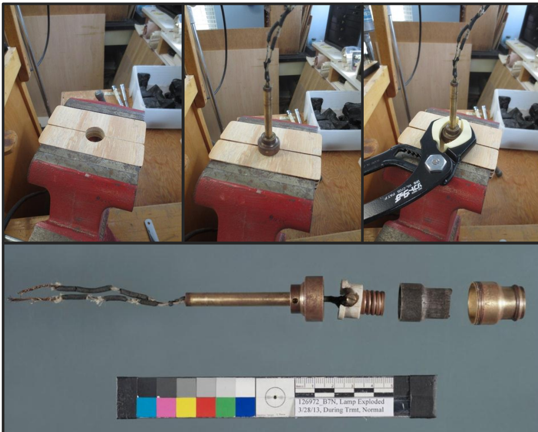
Figure 37: Process used to separate the lamp socket from the shell cap. The upper left image shows the clamp. The center image shows the oiled socket bound by the clamp. The upper right image shows the rubber padded pliers providing the torque necessary to separate the two parts. The lower image is an exploded view of the lamp showing the corroded thread and the degraded wire insulation.
