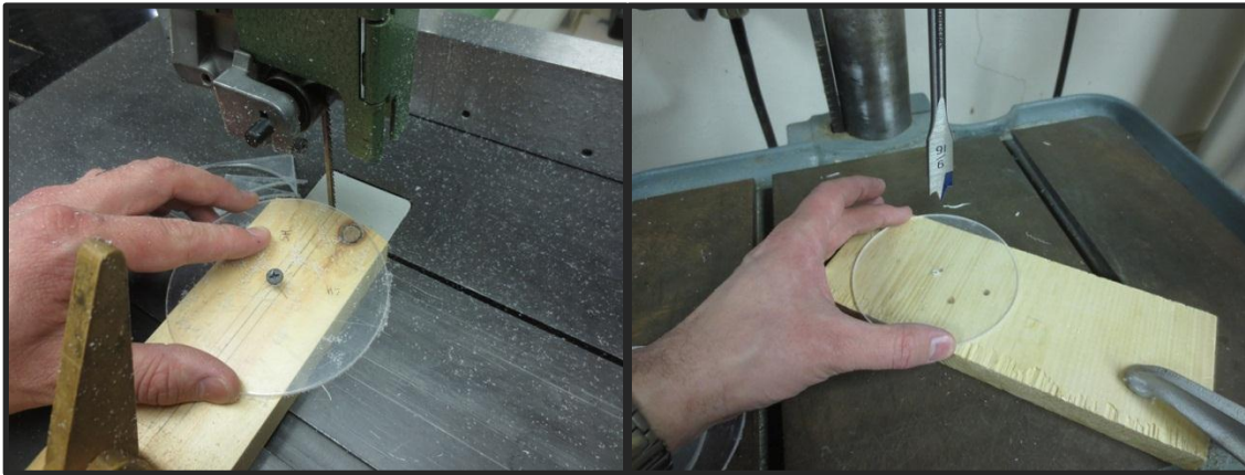
Figure 41: Shaping the acrylic discs on the bandsaw with a simple jig (left), and drilling a hole in the center of the discs with a 9/16" spade bit in preparation for molding.
