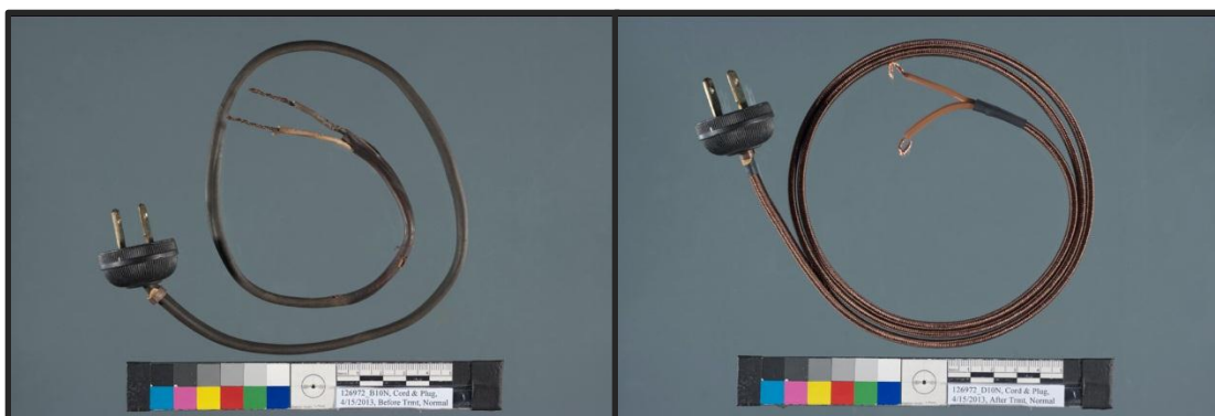
Figure 33: Before (left) and after treatment images of the main power cord, which was replaced with a brown rayon-sheathed two conductor cord. The frayed ends of the rayon, where the sheath was removed to expose the plastic insulator, was managed with rubber heat-shrink tubing.
