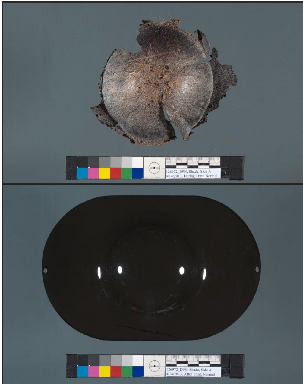
Figure 46: The original, highly degraded cellulose acetate daylight/night discriminator (upper image) compared to its black PMMA replacement.
