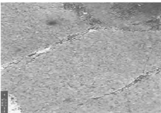
10a. Two microcracks within a quartz grain in granite; both are relatively wide.
