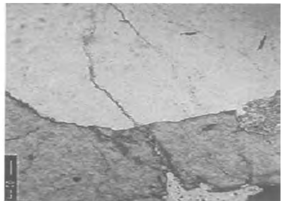
10b: This microcrack extends into multiple grains and is developing numerous offshoots.
