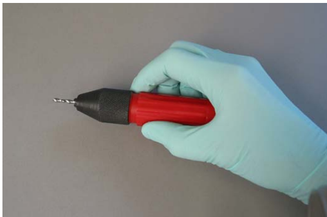
Figure 6. A tungsten bit held in a pin vice can be used to hand drill the inside of a hollow terracotta.
