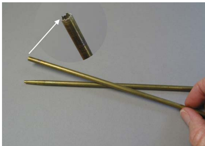
Figure 7. A sampling tube can be used to remove core material from bronzes with very limited access to the interior.
