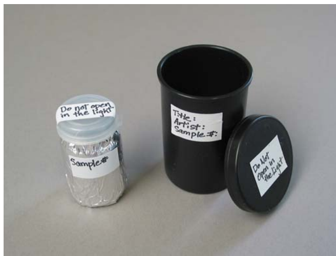
Figure 8. Light-tight sample vials are labeled and weighed before drilling begins.
