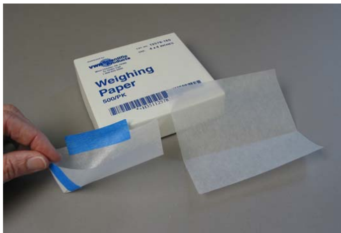
Figure 9. A folded envelope attached inside a hollow sculpture will catch the sample as it is drilled.
